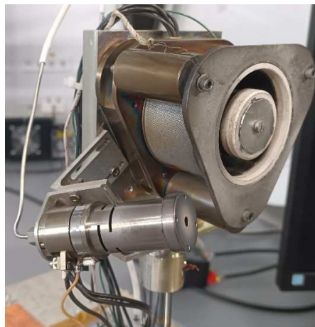
FIGURE 11. General view of the ST-40 Hall thruster.
